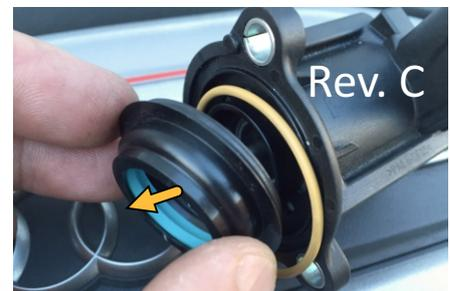
Install the GFB parts onto the solenoid body as shown below, using a little engine oil on the outside of the piston (do NOT use grease or other heavy lubricants). **Make sure to use the GFB supplied spring inside the solenoid coil** – the only factory parts you re-use are the solenoid coil and the yellow o-ring.
